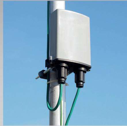
Linkit G1ESDP is a surge discharger for Ethernet protection of digital systems.
